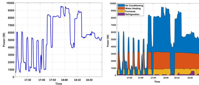
FIGURE 30. Almost real-time household level total power provided by the advanced meter and the desired disaggregated power.
