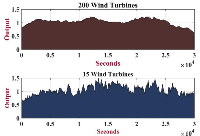
FIGURE 17. Variation in wind energy generation output for 200 and 15 wind turbines placed in dispersed positions.
