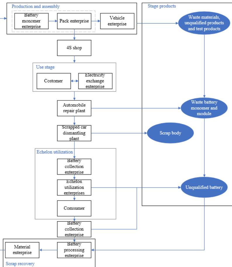
FIGURE 1. Power battery life cycle recovery pipeline process.
