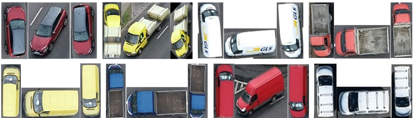
Figure 5. Sample images for automatic detection of a vehicle moving between two cameras.
