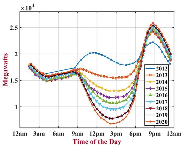
FIGURE 24. Duck diagram interpretation of over-generation risk and ramp requirement.
