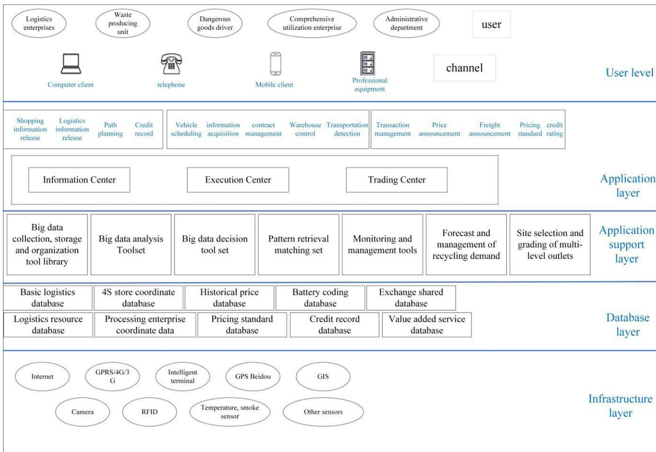
FIGURE 2. Theoretical model of a power battery recovery platform based on big data.
