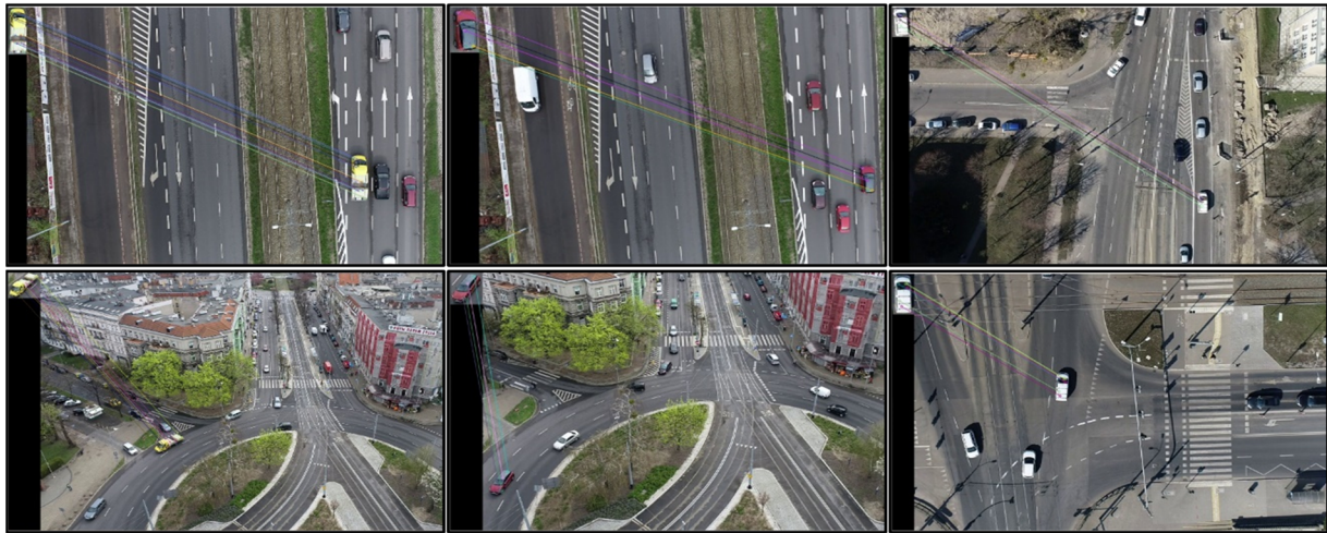
Figure 6. Example results of image analysis for the automatic detection of moving vehicles. Upper image—camera1; Lower image—camera2.
