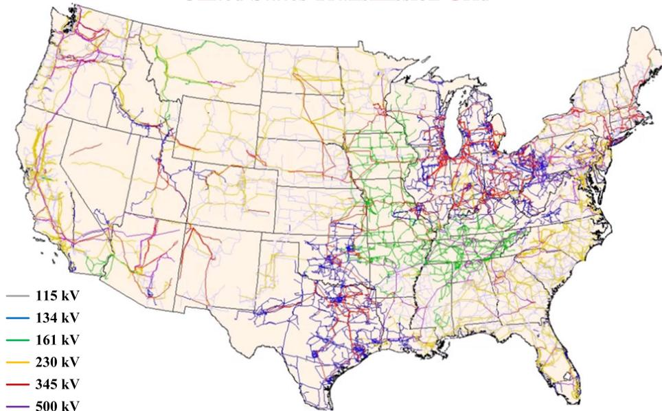
**FIGURE 3.** United States synchronous grid of 186, 411 miles.
